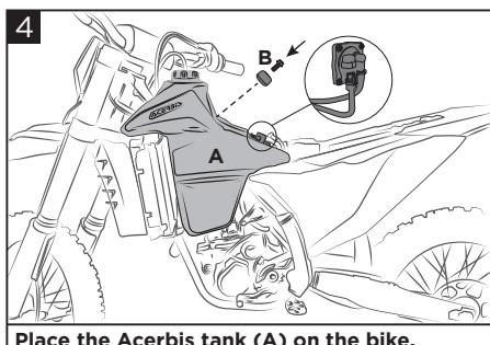
**Place the Acerbis tank (A) on the bike, secure it with the screw + rubber (B) and connect the pump to the connectors.**
