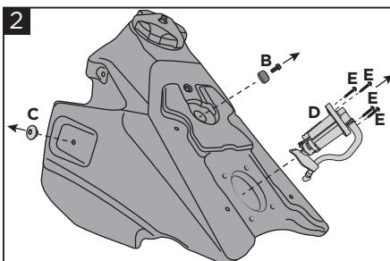
**Remove the original tank, disconnecting the pump connectors and unscrewing the screw and the rubber (B). Completely empty the tank from the petrol and remove the pump (D) through screws (E). Finally remove the screws (C).**
